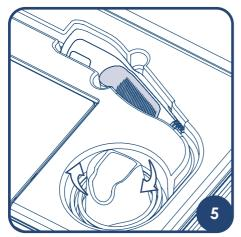
To prevent unnecessary damage, ensure the LumenEye® X1 is packed in the dedicated storage recess and the cable is wrapped in the cable-tidy recess as shown.
