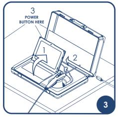
Open the tablet screen to preferred angle (1), connect the LumenEye® X1 to the USB port (2), press the 'power on' button (3) and refer to 'IFU-401' for CHiP software instructions. (Please note: the tablet is controlled via a touch screen interface. Please use the integrated keyboard for typing).
