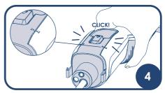
Ensure the manifold is fully in place. An audible click will be heard and the arrows on the manifold will align with those on the LumenEye® X1 handset indicating full engagement.
