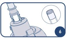
Push the camera cover into the slots firmly until an audible snap is heard. Ensure secure fitting by testing integrity with a gentle pull.
