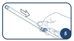
Remove the camera cover from the packaging and slide the connector over the LumenEye® X1 camera tube.
