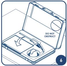
Ensure that the tablet is fully switched off and the tablet screen is placed in the closed position before shutting the case lid. Ensure there is no obstruction of the mount when closing the case lid.
